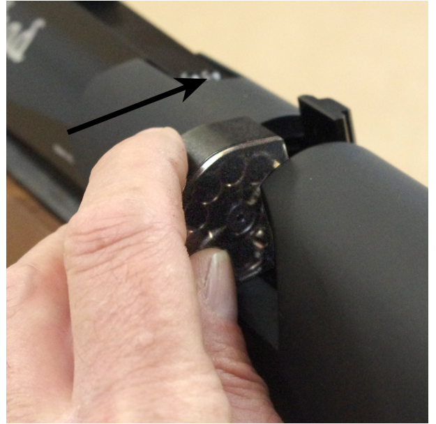
Reload the magazine back into the housing keeping the magazine pressed to the base of the slot.
