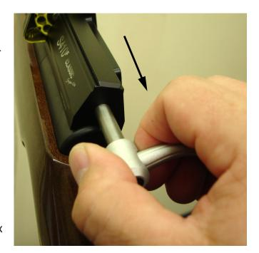
If you find the mechanism has not cocked completely but the magazine has indexed, Re-cock but before closing the bolt, remove the magazine and manually index it back. To the empty chamber.
