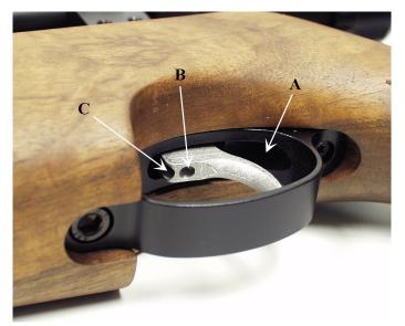
movement increase the weight. Screw (B) & (C) are in the trigger blade itself. Screw (B) adjusts the exact pull-off point. Clockwise decreases the pull-off point. Screw (C) adjusts the length of first stage travel, again clockwise decreases the length of first stage travel.
